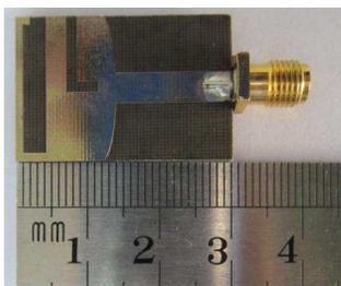
**Figure 5.** Prototype picture of the proposed antenna.
