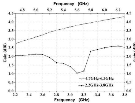
**Figure 8.** Simulated gain of the proposed antenna.
